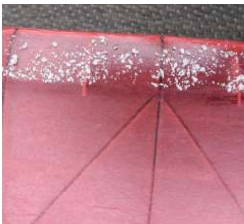
Ben Hobbs' wing upper surface leading edge crazy paving turbulentator
