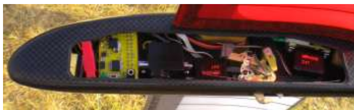
The fuselage of Kraus' F1A, Black Magic timer, Hitec 65HB and Dymond D47 servos
